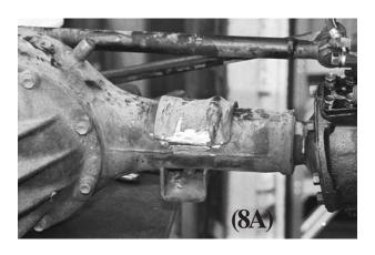
9. Weld the front shock absorber mounts to the existing spring pads as shown below
