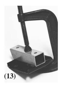
13. Weld the rear bump stop brackets the rear spring plates as shown on the left. Be sure to center the bump stop mount carefully between the holes in the spring plate, this will make it much easier to get a socket on the nuts. (Note: For a neater installation, the old shock absorber mounts may be removed from the spring plates.)
