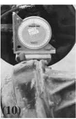
11. Weld the rear absorber mounts to the rear axles as shown . There should be a space between the spring saddle pad and the shock mount of 1 1/4". The pin on the shock mount should be tilted up about 5-10 degrees.
